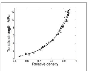
Figure 1. Typical Tensile strength vs Relative density. Note that Porosity = 1 - Relative density. For example, 2% Porosity corresponds to 98% Relative density. Tensile strength or hardness is measured by diametrical compression, (from IJP 484, 29-37).
