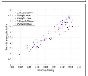
Figure 2. Tensile strength vs Relative density for a formulation with different amount of Magnesium Stearate (lubricant) and different mount of mixing in seconds. (from Powder Technology, 336, 360-37)
